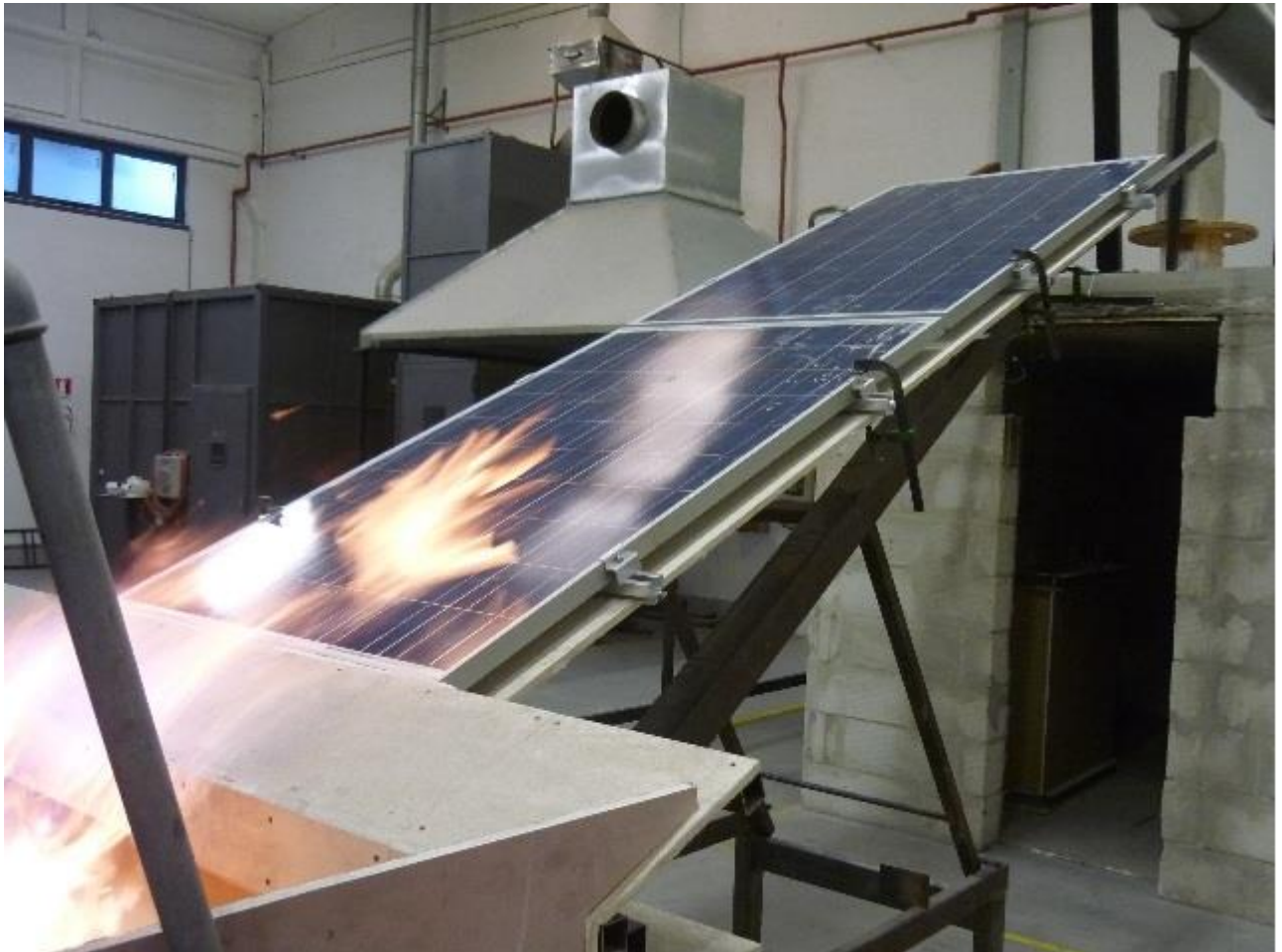
Figure 13 – Spread-of-flame test (LAPI laboratory)
