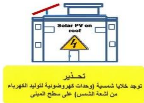
Figure 20 – Sign to be used to indicate the presence of a PV plant
