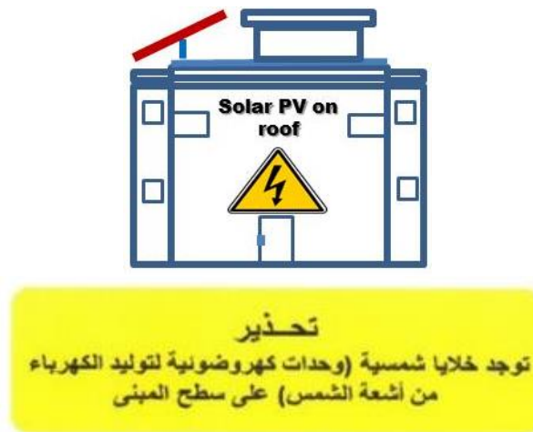
Figure 14 – Signs to be used to indicate the presence of a PV plant
